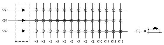
Note: In this circuit, pressing three or more times may cause the OFF switches to be determined as being ON.
