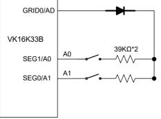
Note: A1-A0 float is 0, connect is 1, when all float the device address is 0xE0
