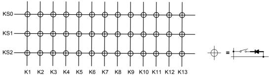
When pressing twice is assumed,KS0-KS2 is required to connect diodes in series, shown as below:
