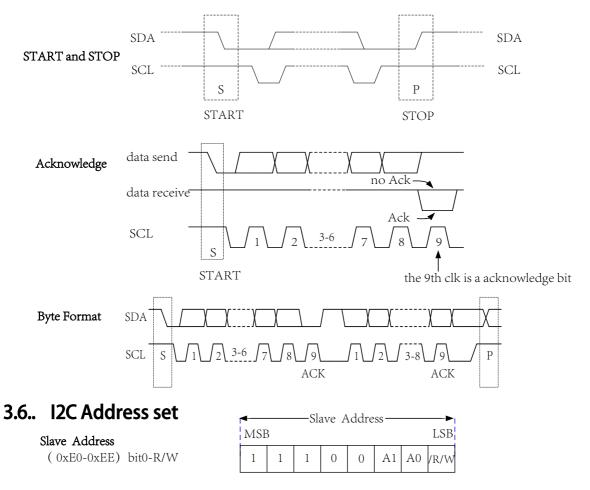
I2C slave address is selected through A2-A0 pins, and I2C slave address is updated during power <u>on reset or key s</u>canning cycle, shown as below :
