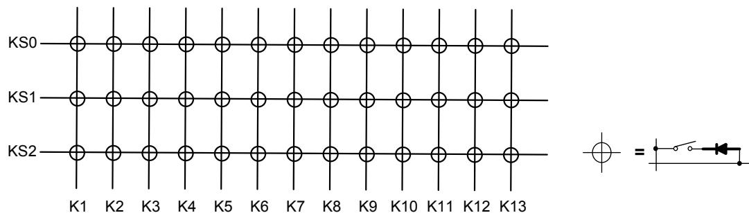
When pressing twice is assumed, KS0-KS2 is required to connect diodes in series, shown as below:
