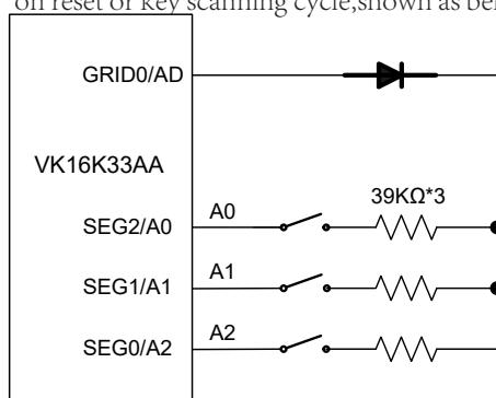
Note: A1-A0 float is 0, connect is 1, when all float the device address is 0xE0
