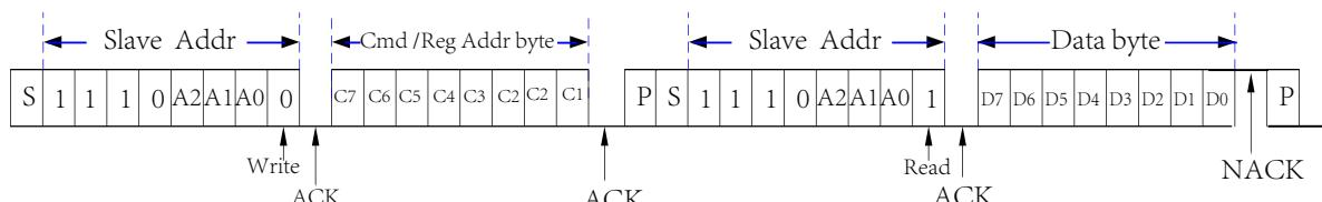
Read n bytes data. The address pointer will auto-increase after received ACK. When reading the key, read 6 data continuously from start address 0x40.
