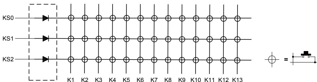
Note: In this circuit, pressing three or more times may cause the OFF switches to be determined as being ON.
