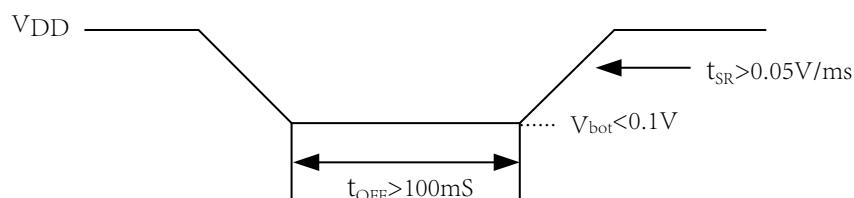
When power on, NC pin is high-level and POR is disable. In order to make the internal circuit in the reset state, it must be configured as follows:
