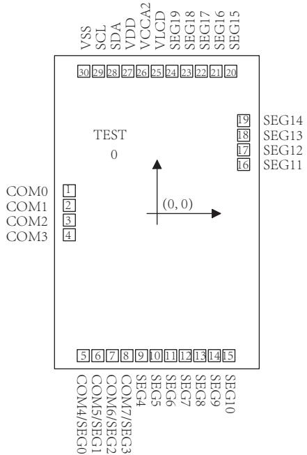
Chip size: 1150×1715 um<sup>2</sup>      Substrate: connected to VSS
